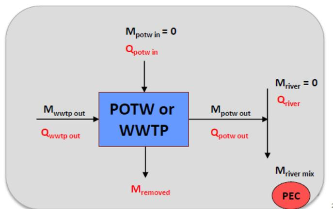
Figure 5 Mass balance of wastewater treatment steps
