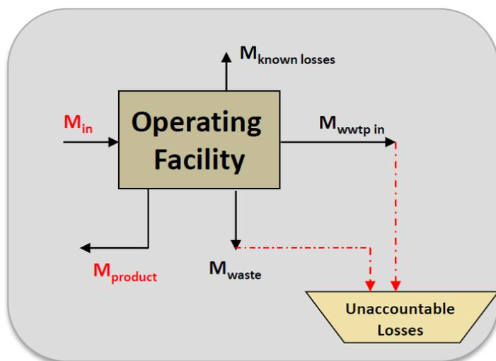
Figure 7 Mass balance of the operating facility
